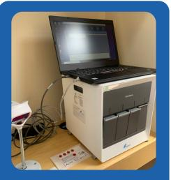
GeneXpert Cepheid machine = finger prick of blood into a machine - tests for active hepatitis C RNA in 60 minutes
